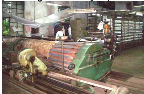
(1) Winding the yarn thread onto the warp beam
