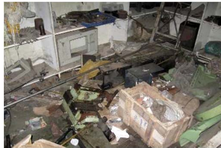
No protection to prevent damage and rust
